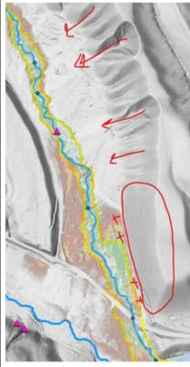
Red arrows indicate area upvalley where landsliding has occurred. The southern end of this geologic formation (red circle) has not had these type of failures. Houses exist at the toe of this slope (approximated by red "x").
